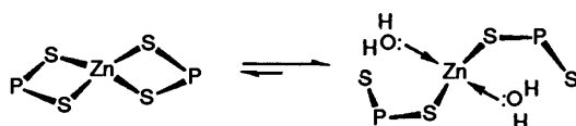
Figure 5. Schematic representation of the co-ordination of water to 'normal' \text{Zn}[\text{S}_2\text{P}(\text{OPr}')_2]_2 ; alkoxy groups attached to phosphorus have been omitted.
